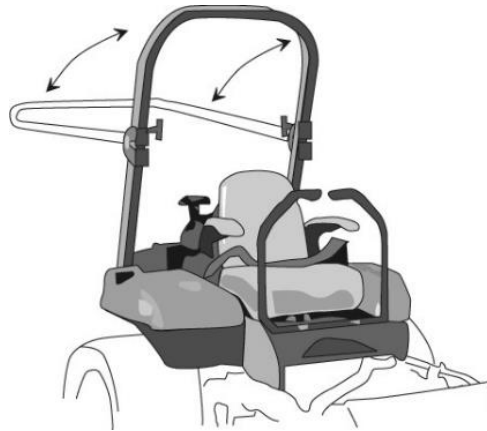
Figure 2 – Example of roll-over protection structures (ROPS) fitted to a ride-on mower
