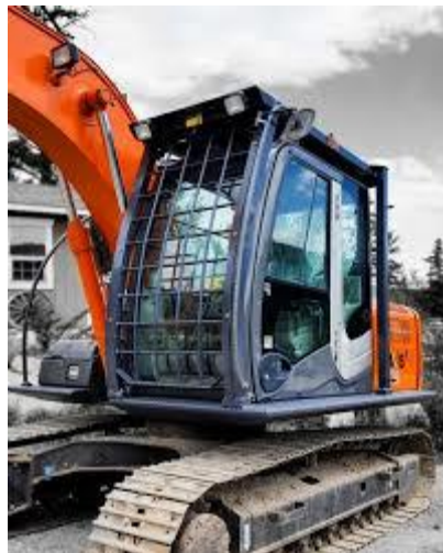
Figure 1 – Example of falling object protective structure (FOPS) fitted to excavator cabin
